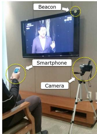
**Figure 1.** A prototype of Smart TV logging system
