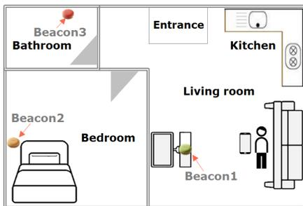
**Figure 2.** The deployment of Beacons for the trial study
