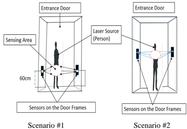
Figure 3: Paired laser Sensors at knee and shoulder positions
